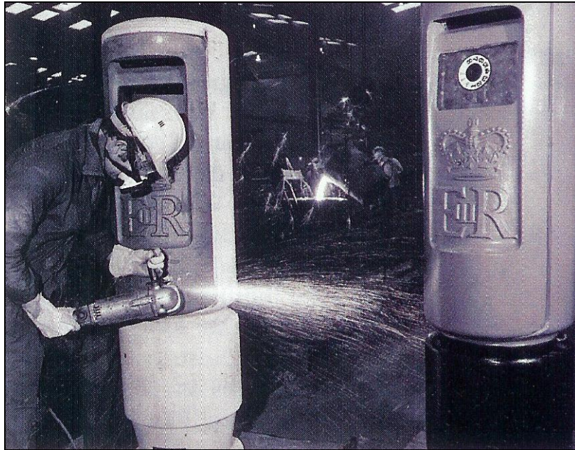
Grinding the K box door casting
