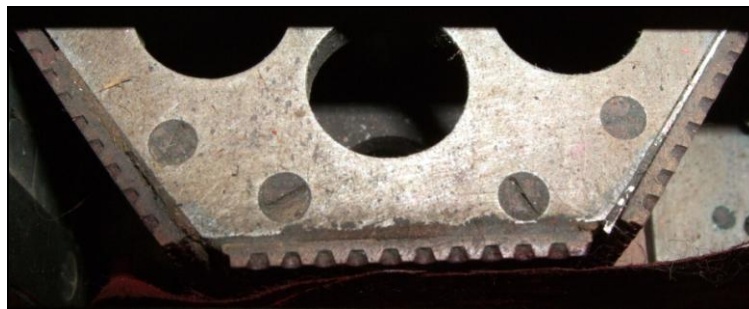
The three postage dies seen from above. Note the 'perforated' top edges to the steel dies.
