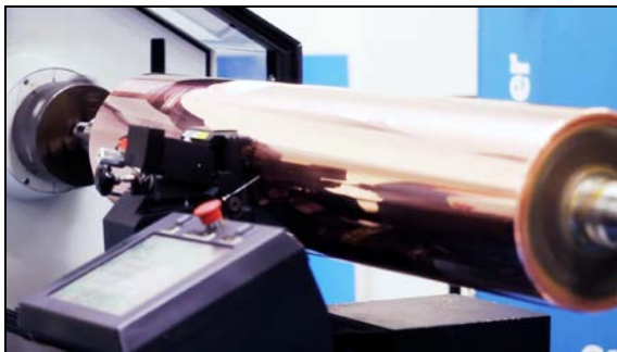
Fig 4 The Hommel Tester taking measurements of the intentionally scratched cylinder. Image © Saueressig Ltd.
