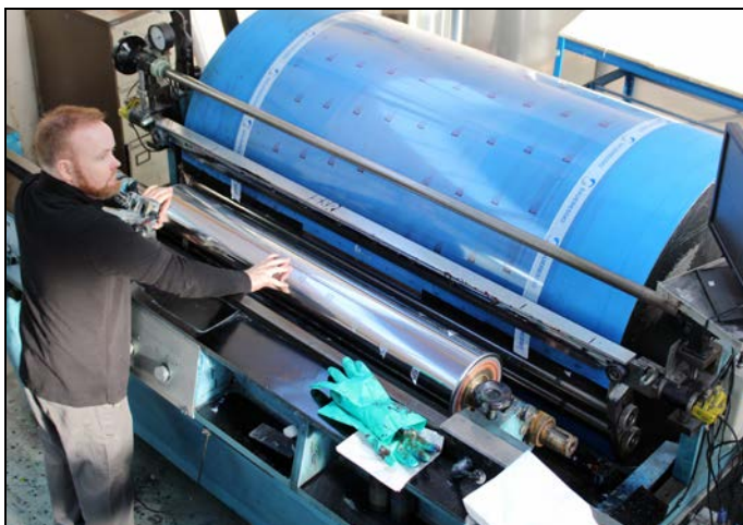
Fig 10 The single colour Heaford proofing press. Image © Saueressig Ltd.
