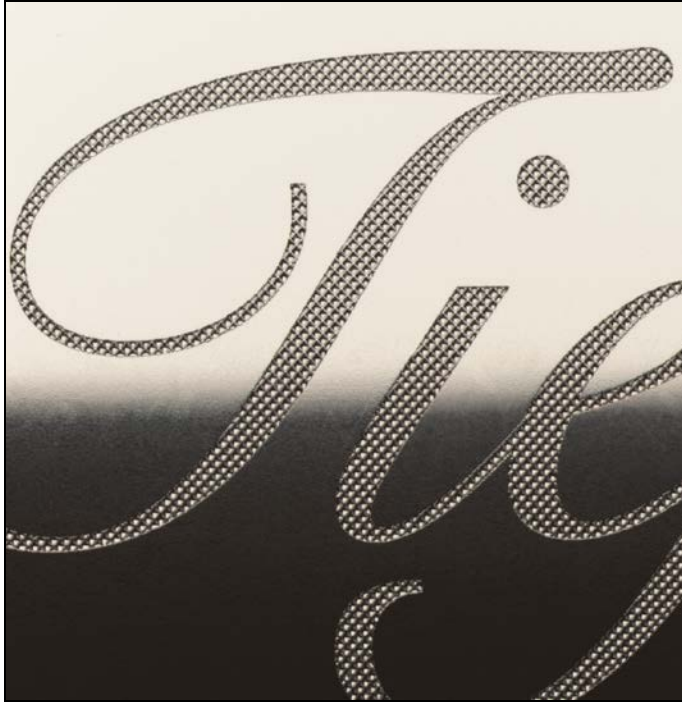
Fig 9 Detail from a Saueressig gravure cylinder that has been chromed.
